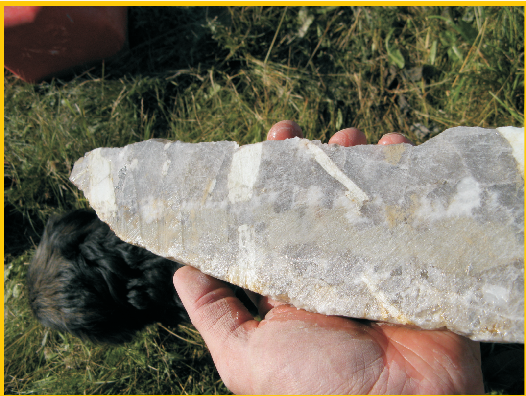
Figure 11b. White laths of spodumene with feldspar, quartz and muscovite. International property, Bouvier showing. UTM Coord.: Easting: 714525; Northing: 5370634; NAD83; Zone 17N.
